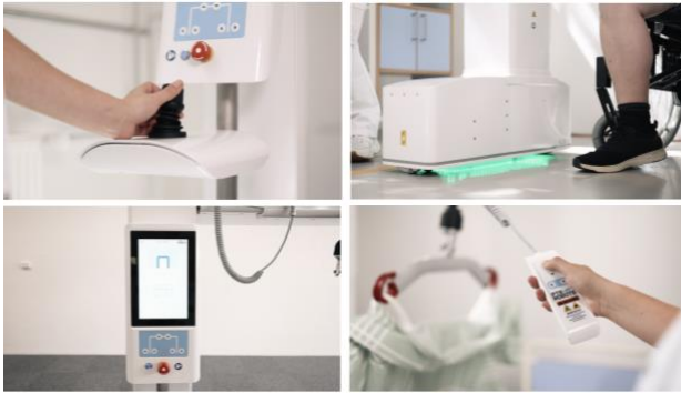
Figure 2. Top left: joystick to control robot movement. Top right: Omnidirectional wheels. Bottom left: Screen and panel to control traverse. Bottom right: remote control to operate lifting hoist
